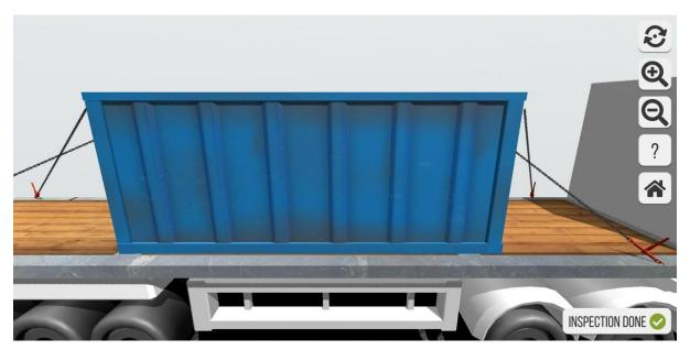
**Hidden errors:** Container: Not enough straight lashings. BOTH backward spring lashings: Lash has a faulty angle. BOTH forward spring lashings: Lash is not correctly pre-tensioned. One forward spring lashing: Chain is worn and could break
