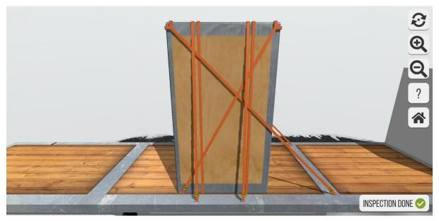
**Hidden errors:** Forward direction spring lashing: Lash is worn and could break. Backward direction spring lashing: Lash has a faulty angle
