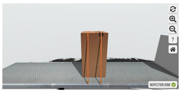
Hidden errors: Paper box: Not enough top-over-lashings. One top-over lashing: Edge protection is missing
