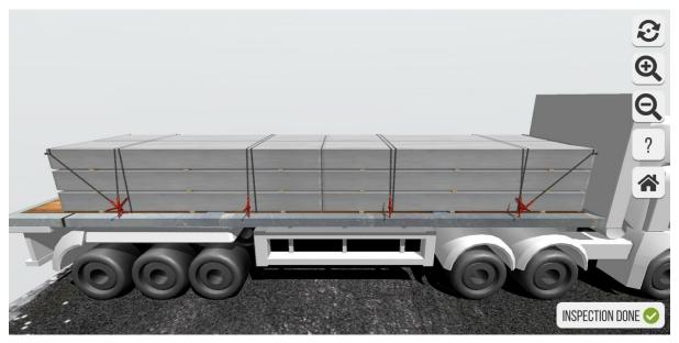
*Hidden errors:* Backward chain spring lashing: Chain is worn and could break. Forward concrete elements: Not blocked against head board
