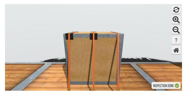
**Hidden errors:** Forward top-over lashing: Edge protection is missing. Wooden box: Not enough top-over-lashings
