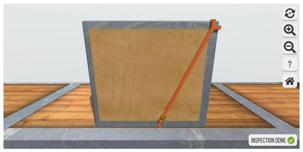
**Hidden errors:** Wooden box: Needs spring lashing. Spring lashing: Lash has a faulty angle. Spring lashing: Lash is worn and could break
