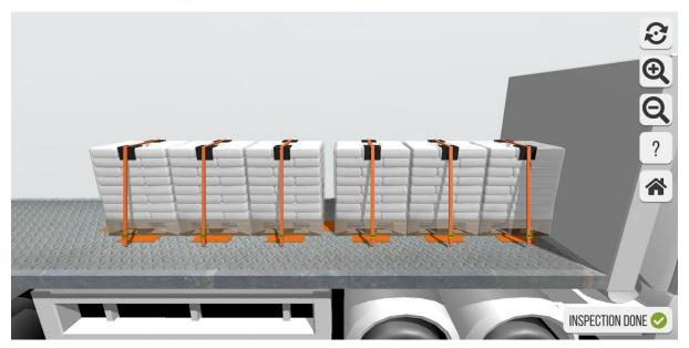
**Hidden errors:** Second pallet from front top-over lashing: Lash has cuts and could break. Third pallet from front: Too much space between cargo items. Fourth pallet from front: Too much space between cargo items
