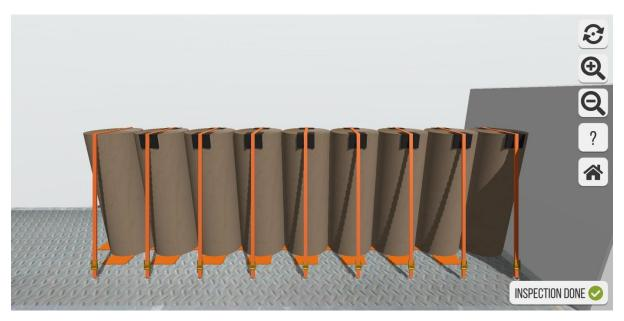
**Hidden errors:** First paper roll from front: Needs friction mats. Last paper roll from front topover lashing: Edge protection is missing
