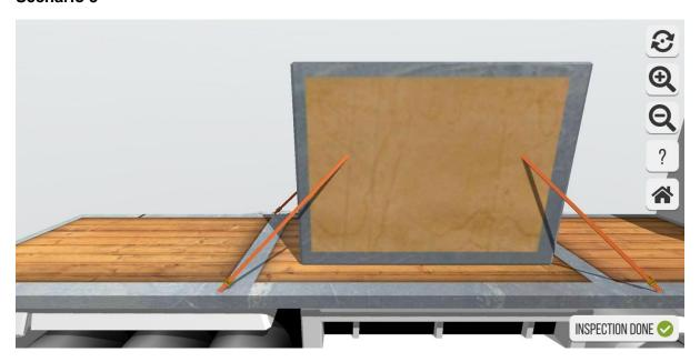
**Hidden errors:** Backward right straight lashing: Lash label is missing. Forward right straight lashing: Lash is worn and could break. Wooden box: Lashings are too weak
