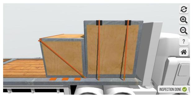
**Hidden errors:** Forward box: Not blocked against head board. Backward box spring lashing: Lash label is missing
