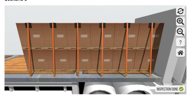
Hidden errors: Third top-over lashing from the back: Lash is not correctly pre-tensioned
