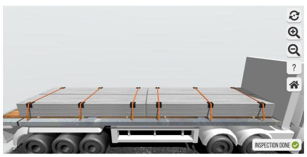
**Hidden errors:** BOTH concrete stacks: Faulty underlays. Forward concrete stack: Not blocked against head board
