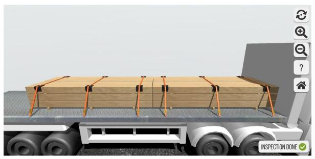
**Hidden errors:** BOTH timber stacks: Faulty underlays. Forward timber stack forward top-over lashing: Lash label is missing. Back timber stack forward top-over lashing: Lash is worn and could break
