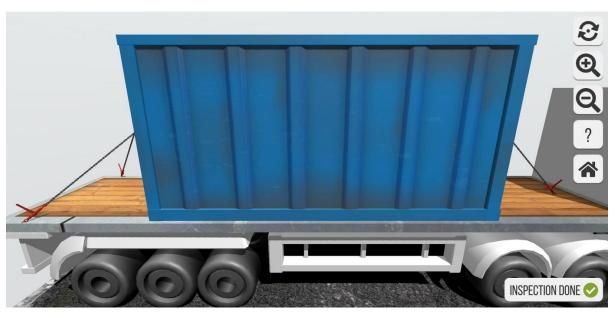
**Hidden errors:** Container: Not enough straight lashings. One backward chain: Chain is worn and could break. Forward chain: Lash is not correctly pre-tensioned
