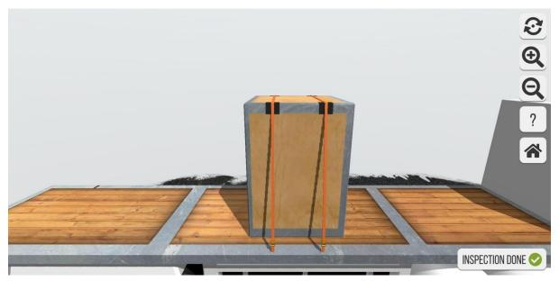
Hidden errors: Wooden box: Not enough top-over-lashings. One top-over lashing: Lash is worn and could break
