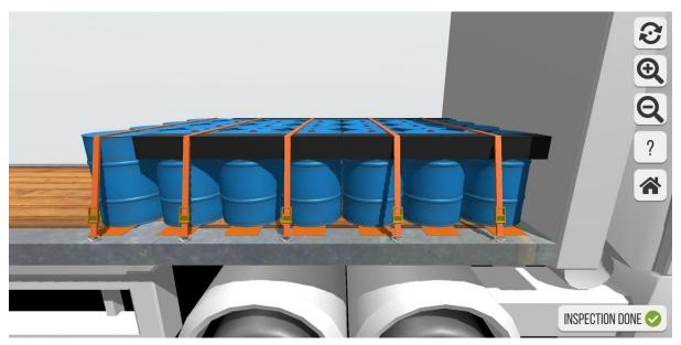
**Hidden errors**: Back row: Needs spring lashing. Back row top-over lashing: Edge protection is missing
