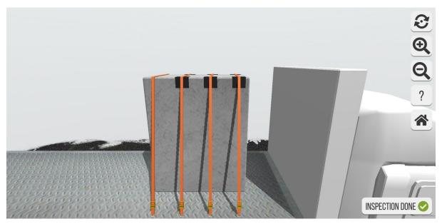
**Hidden errors:** Backward top-over lashings: Edge protection is missing. Concrete object: Not enough top-over-lashings
