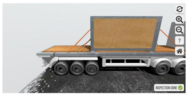
**Hidden errors:** Backward right direction straight lashing: Lash has a tied knot. Wooden box: Not enough straight lashings
