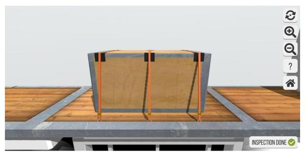
**Hidden errors:** Wooden box: Not enough top-over-lashings. One top-over lashing: Lash is not correctly pre-tensioned. One top-over lashing: Lash label is missing
